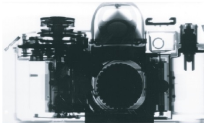
X-ray image of a film SLR camera
