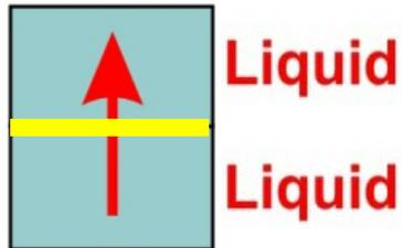
Membrane is immersed in liquid water. Pressure is applied on one side to create hydraulic pressure driven permeation.
