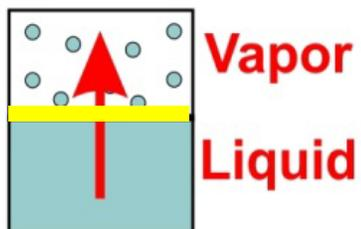
Membrane is floated on liquid water. Humidified air is flowed on one side to create concentration gradient driven permeation.
