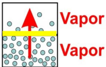
One side of the membrane is exposed to saturated water vapour. Humidified air is flowed on one side to create concentration gradient driven permeation.
