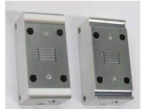
Parallel channels (internal manifolds, Macor® spacers)
