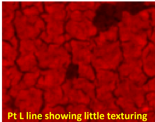
Pt L line showing little texturing Overall loading Pt/cm 2 uniform, identical to baseline MEA
