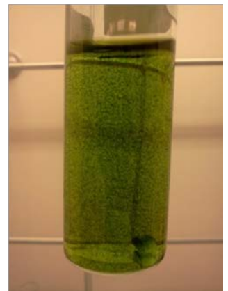
(Left) Nine metal salt precursor solutions with iron to cobalt ratios shown in Table (Cobalt only on left and Iron only on right). (Right) The iron only solution during polymerization of the polyaniline.
