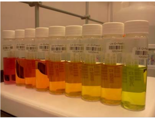
(Left) Nine metal salt precursor solutions with iron to cobalt ratios shown in Table (Cobalt only on left and Iron only on right). (Right) The iron only solution during polymerization of the polyaniline.
