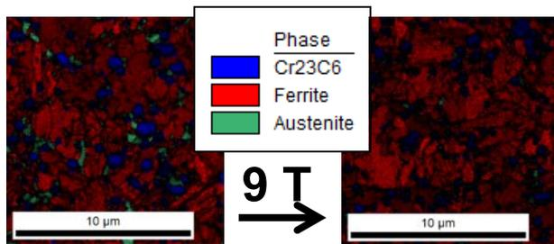
Processing steel in a 9 Tesla magnetic field minimizes retained austenite.
