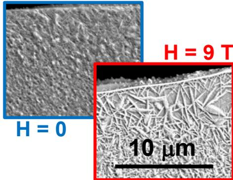
Crystallizing ferromagnetic alloy in a magnetic field changes grain morphology (SEM).
