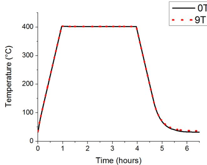
Kapton<sup>®</sup> roll-good stable under Ar and H<sub>2</sub> at 400°C
