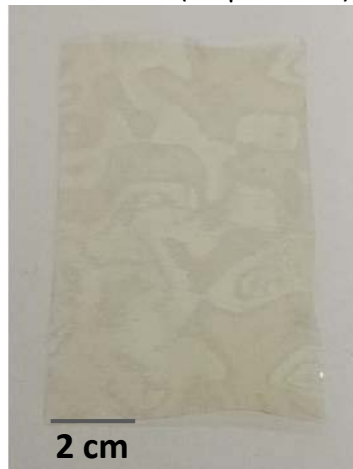
ATM-PP (60 \mu\text{m} thick)
