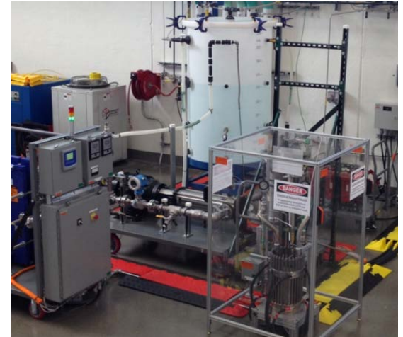
NREL electrolysis grid-integration test bed
