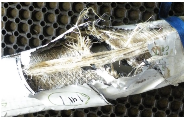
Burst Test Failure
