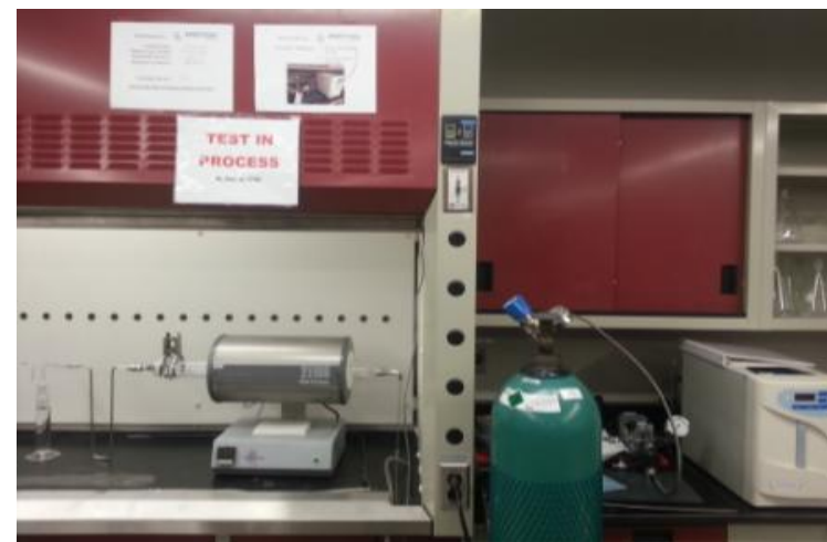
Safety-qualified hydrogen reducing furnace
