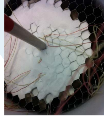
MOF loading in hex-cells
