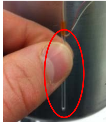
Glass capillary tube used to control TC location
