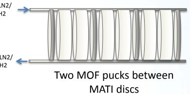
Disc = 1x etched + 1x un-etched plate
