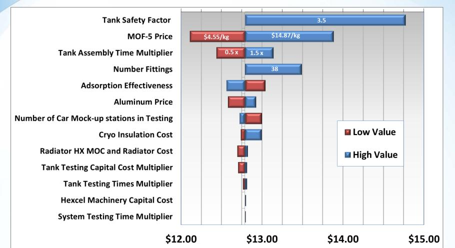
Hexcell H2 Adsorbent Storage System Cost (\$/kWh)
