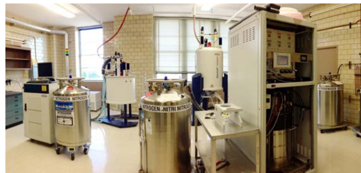
Sievert's type apparatus (PCTPro-200, HyEnergy, LLC) with extended pressure and residual gas analysis (RGA) capabilities
