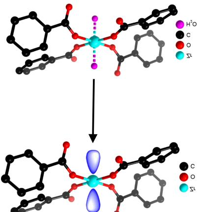
Proposed Work– Improving Adsorption Enthalpy through Unsaturated Metal Center (UMCs) in MOF by ALD
