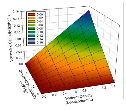
Volumetric capacity & thermal conductivity can be improved by compounding MOFs with engineered carbon (EC)
