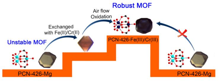
Through a sequential methathesis of labile metals and subsequent oxidation stable crystalline high valent MOFs have been obtained
