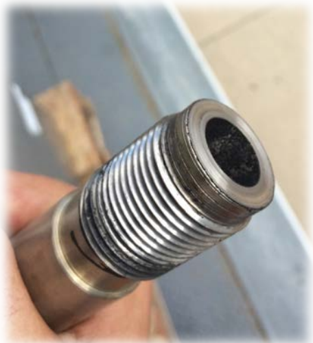
Contaminant in hydrogen line
