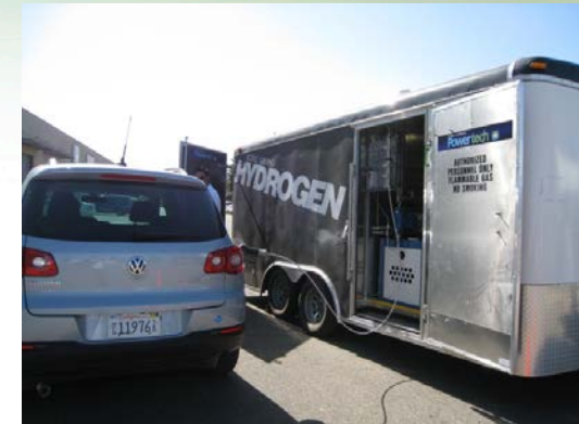
Example of mobile H2 system from Powertech
