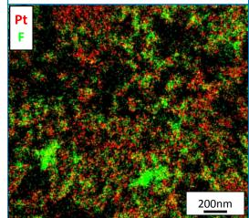
Non-homogeneous ionomer distribution: dependent on density of Pt/C agglomerates and association with porosity
