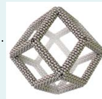
Pt 3 Ni Nanoframes/C with Pt-skin surfaces
