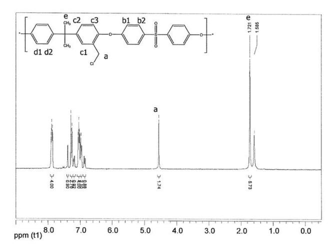
Ratio of "a" to "e" allows degree of chloromethylation Mano Sonic
