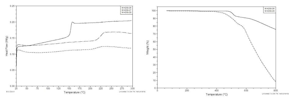
Glass transition temperature of copolymer depend on comonomer selection and ratio. Some polymers are semi-crystalline.
