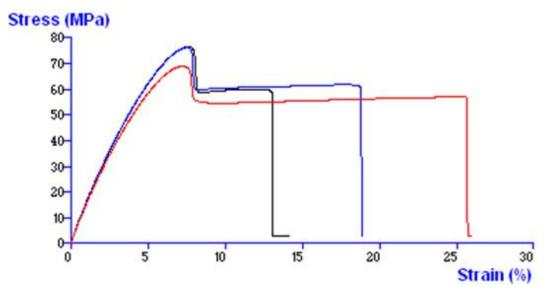
Modulus: 1600-2800 MPa Tensile Strength: 70-90 MPa Percent Elongation: 3-10
