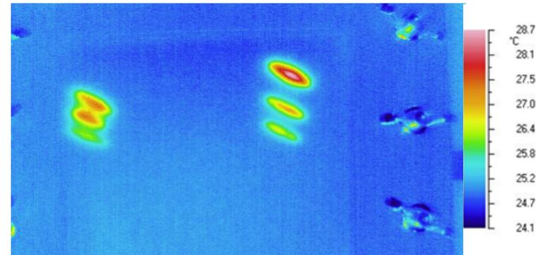
GM GDE + membrane half cell with cuts in membrane prior to lamination, tested at 0.5 lpm  $\text{H}_2$  and 5 sec pulse: 3  $^{\circ}\text{C}$  temperature rise
