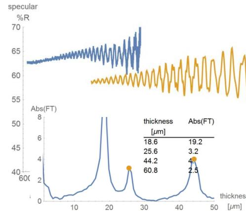
Visible and IR reflectance spectroscopy for 25  $\mu\text{m}$  Nafion with 2 protective layers
