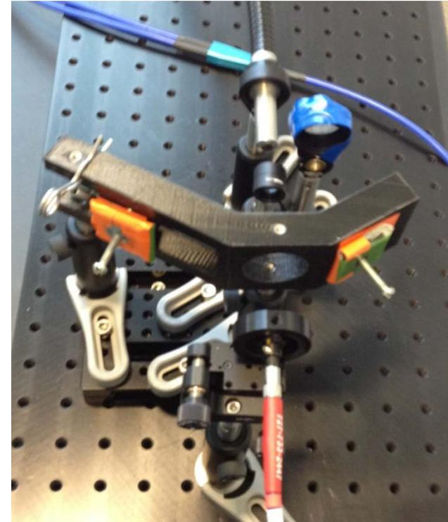
Single-point fast spectroscopy test-bench with broadband light source, focusing optics, specimen holder, receiving optical fiber and Si and InGaAs spectrometers (not shown); Spot size:  $\sim 10 \text{ mm}^2$
