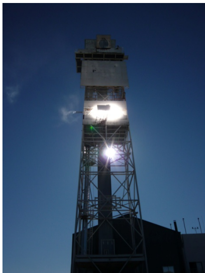
DLR 100 kW Solar H 2 Receiver
