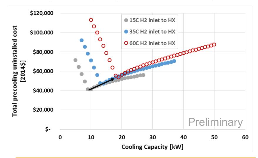
J-T temperature increase must be mitigated before inlet to precooler HX
