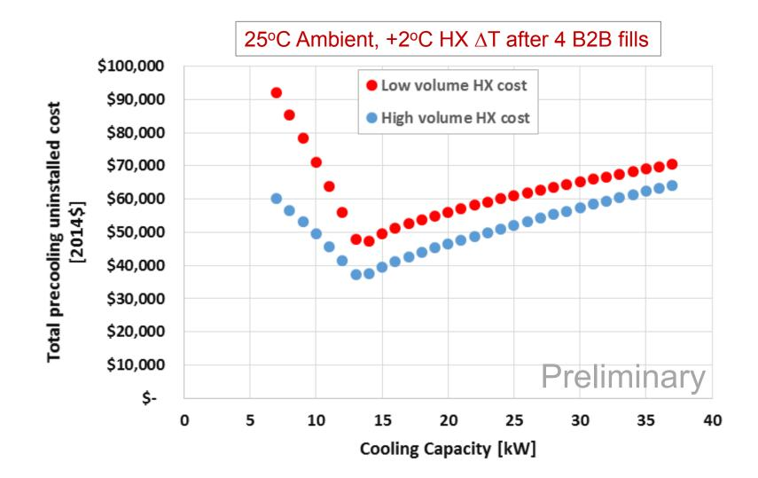
Needed to estimate potential for cost reduction of current HX technology with mass production
