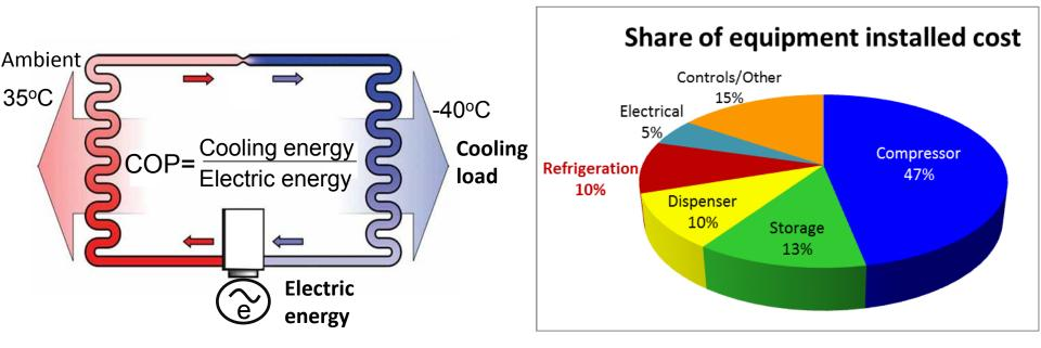
Equipment cost of refrigeration unit plus heat exchanger (HX) is significant
