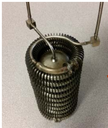
Coiled-fin tube exchanger in CHEX between dual AMRs
