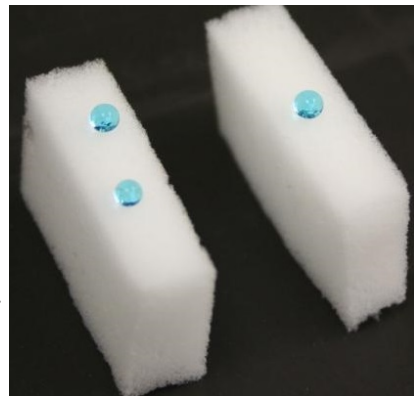
3. Water droplets bead up on the cross-sectioned foam, demonstrating the hydrophobic coating has penetrated deep into the foam.
