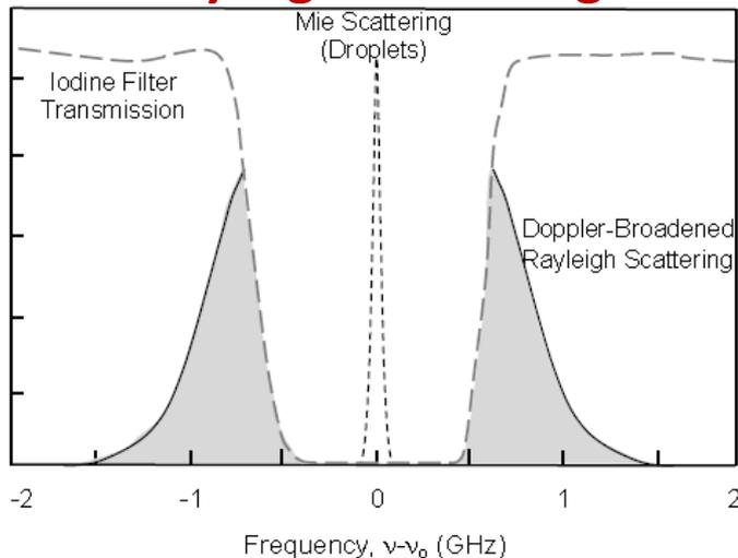
Using a narrow band-width ( $\Delta\nu < 0.003 \text{ cm}^{-1}$ ) laser and a molecular I<sub>2</sub> filter tuned to center wavelength of the laser beam, it is possible to filter out the Mie scattered light
