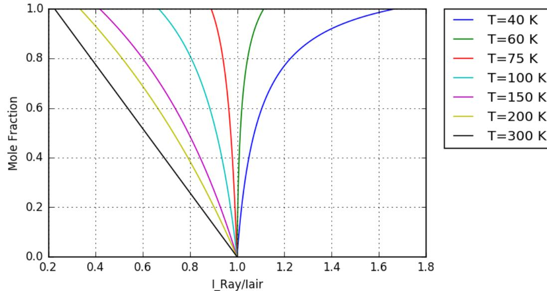
**Rayleigh signal between air and H<sub>2</sub> is indistinguishable in the temperature range 60 – 75 K**
