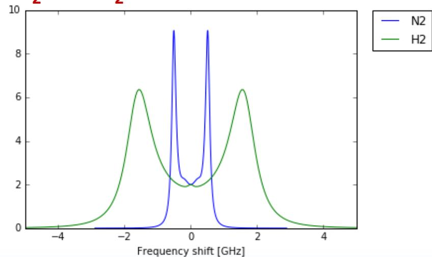
Doppler broadened H<sub>2</sub> spectra is promising for filtered Rayleigh scattering measurements
