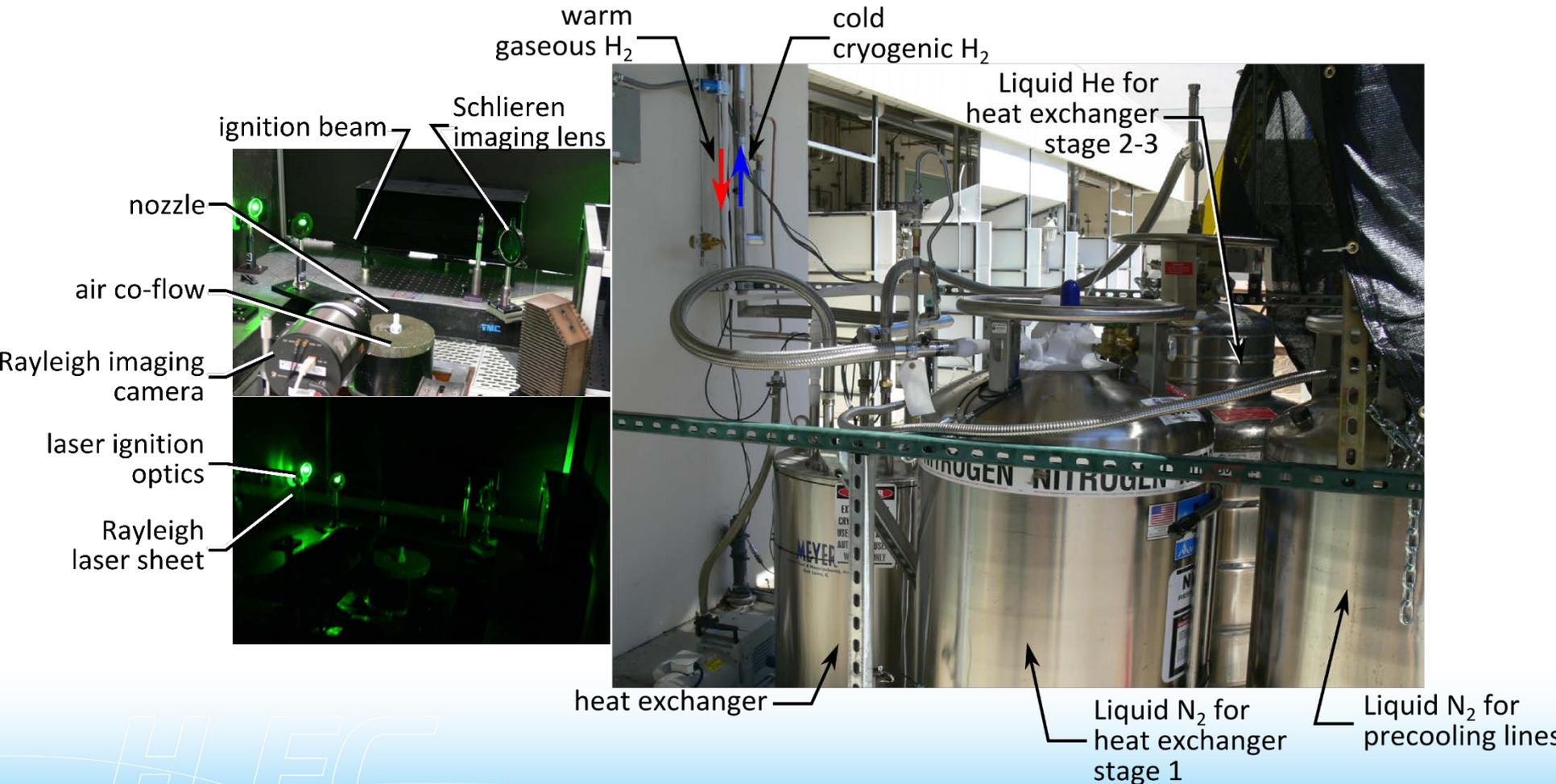
➤ Multiple diagnostics are used to precisely characterize releases
