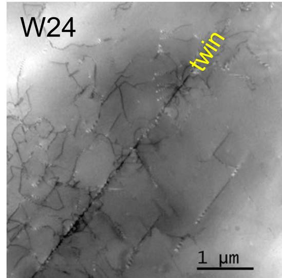
Strong crystallographic alignment of dislocation lines along {111} planes.
