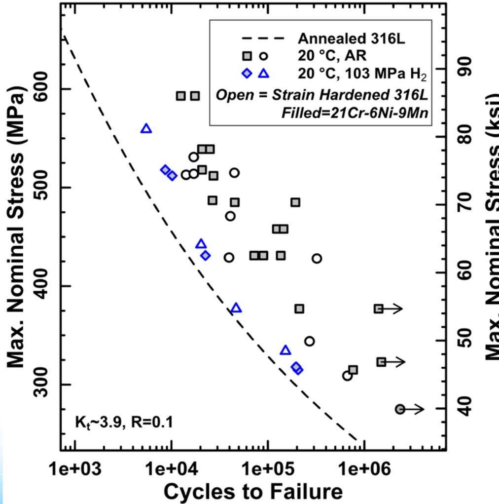
**Fatigue life is longer for both the strain hardened 316L and XM-11 compared to the annealed 316L steel**
