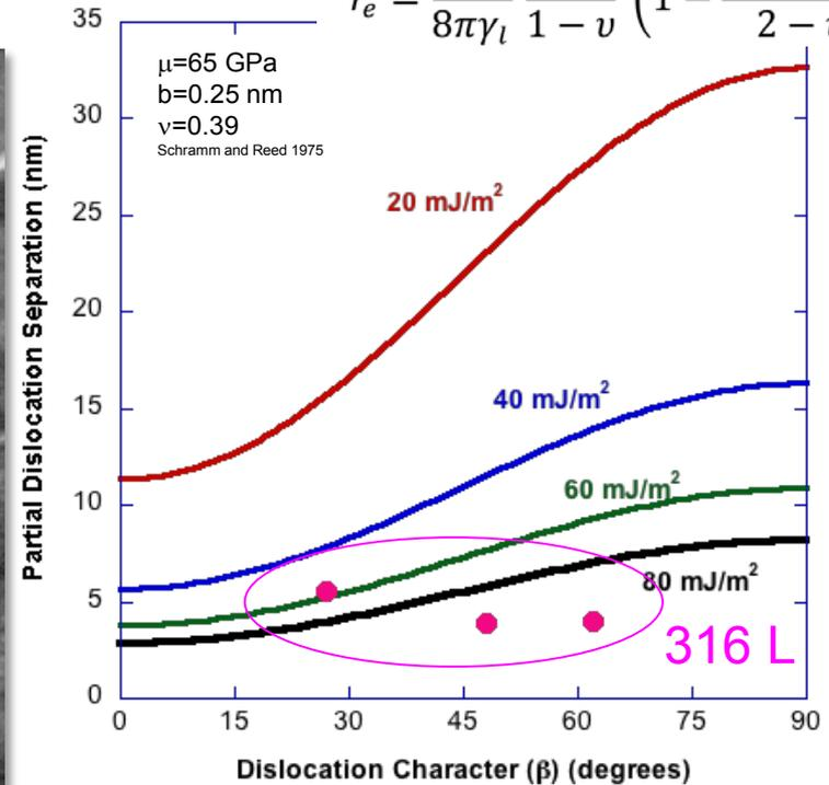
Initial measurements on 316L give **SFE ~60-100 mJ/m<sup>2</sup>**
