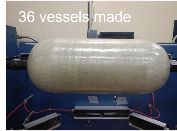
Vessel winding Hexagon Lincoln
