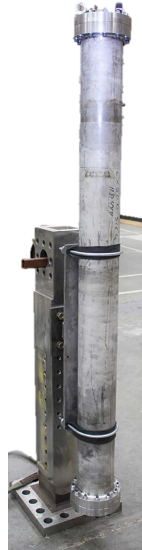
Actual safety containment vessel with stand
