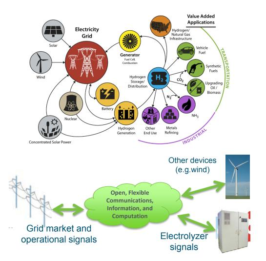
Project connects real-time grid simulator at INL with electrolyzer testbed at NREL to test capabilities to absorb curtailed renewable energy.
