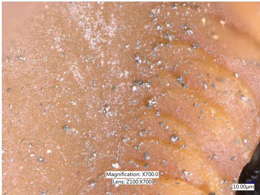
Seat material from a valve exposed to pre-cooled hydrogen. Metal flakes visible near fracture.
