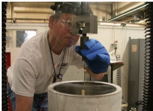
Cold strength test of candidate liner materials
