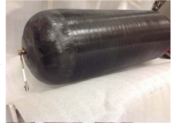
Cryogenic vessel designed for 6400 cycles (1600 cycles, safety factor=4)
