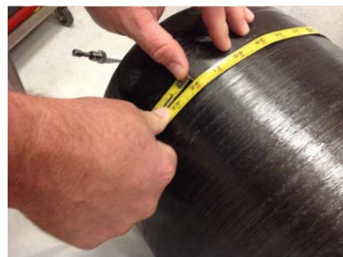
First thin-lined (1.8 mm) vessel, 81% volumetric efficiency (vs. 70% conventional vessels)
