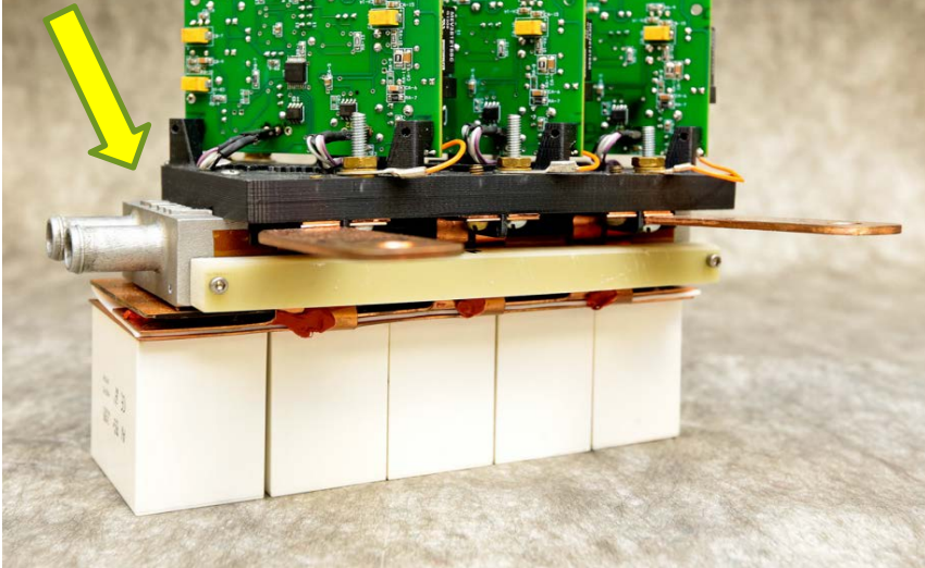
ORNL 3D printed power module design
