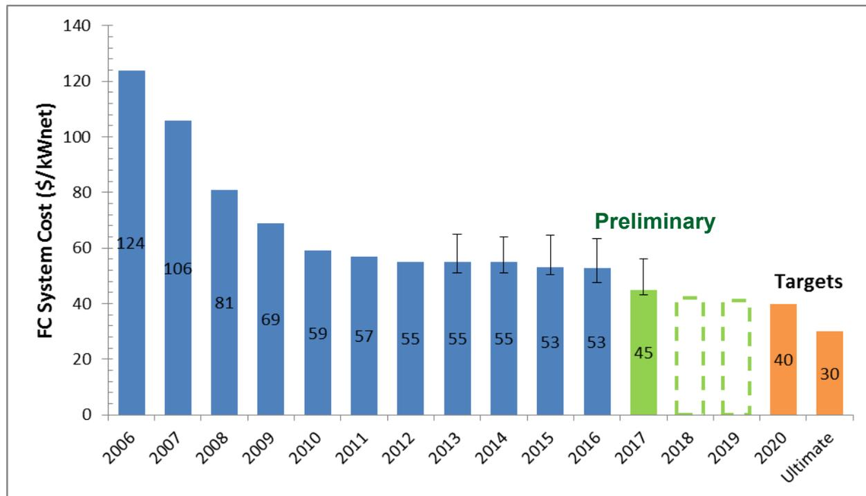
**Preliminary values for 2017 fuel cell transportation system cost at volumes of 500,000 and 100,000 units/year are \$45/kW and \$50/kW, respectively.**
