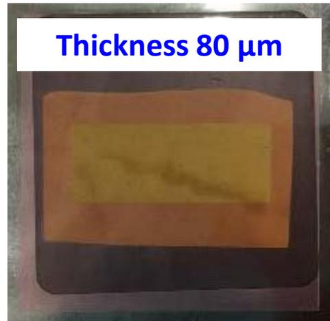
Hot-pressed membrane with sub-gasket
