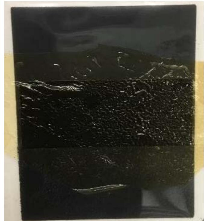
20 micron Membrane on top of the sub-gasket
