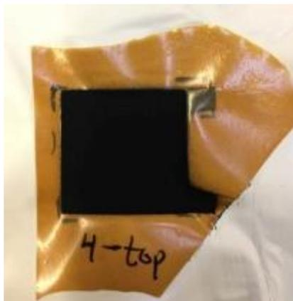
**Stand alone film after 20,000 wet/dry cycles, accelerated stress test.**
