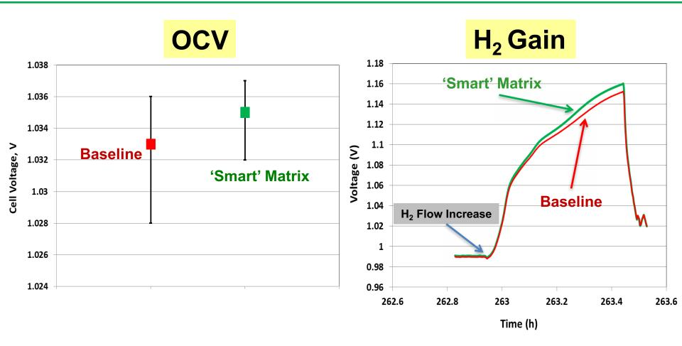
BOL\* open-circuit voltage (OCV) and H<sub>2</sub>-gain tests confirmed improved gas sealing efficiency of 'Smart' Matrix.
