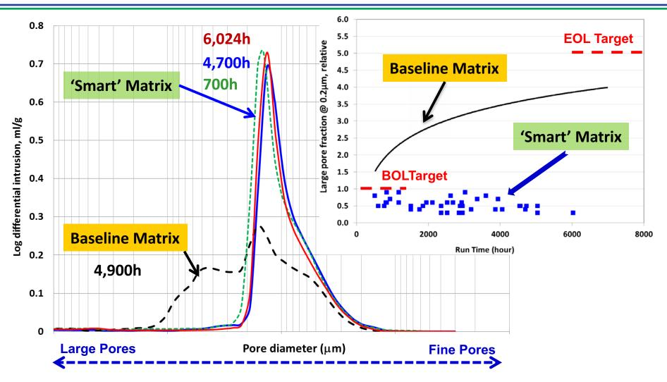
□ Projected meeting EOL\* pore-structure target (<50% of pores >0.2µm in 10 years) in accelerated cells
