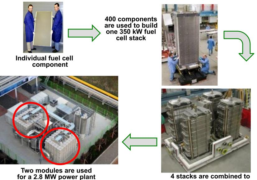
4 stacks are combined to build a 1.4 MW modules
