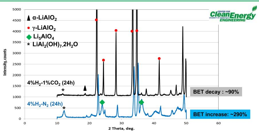
Hydroxide promotes forming fine intermediates: α-Li<sub>5</sub>AlO<sub>4</sub> and LiAl<sub>2</sub>(OH)<sub>7</sub>-2H<sub>2</sub>O
