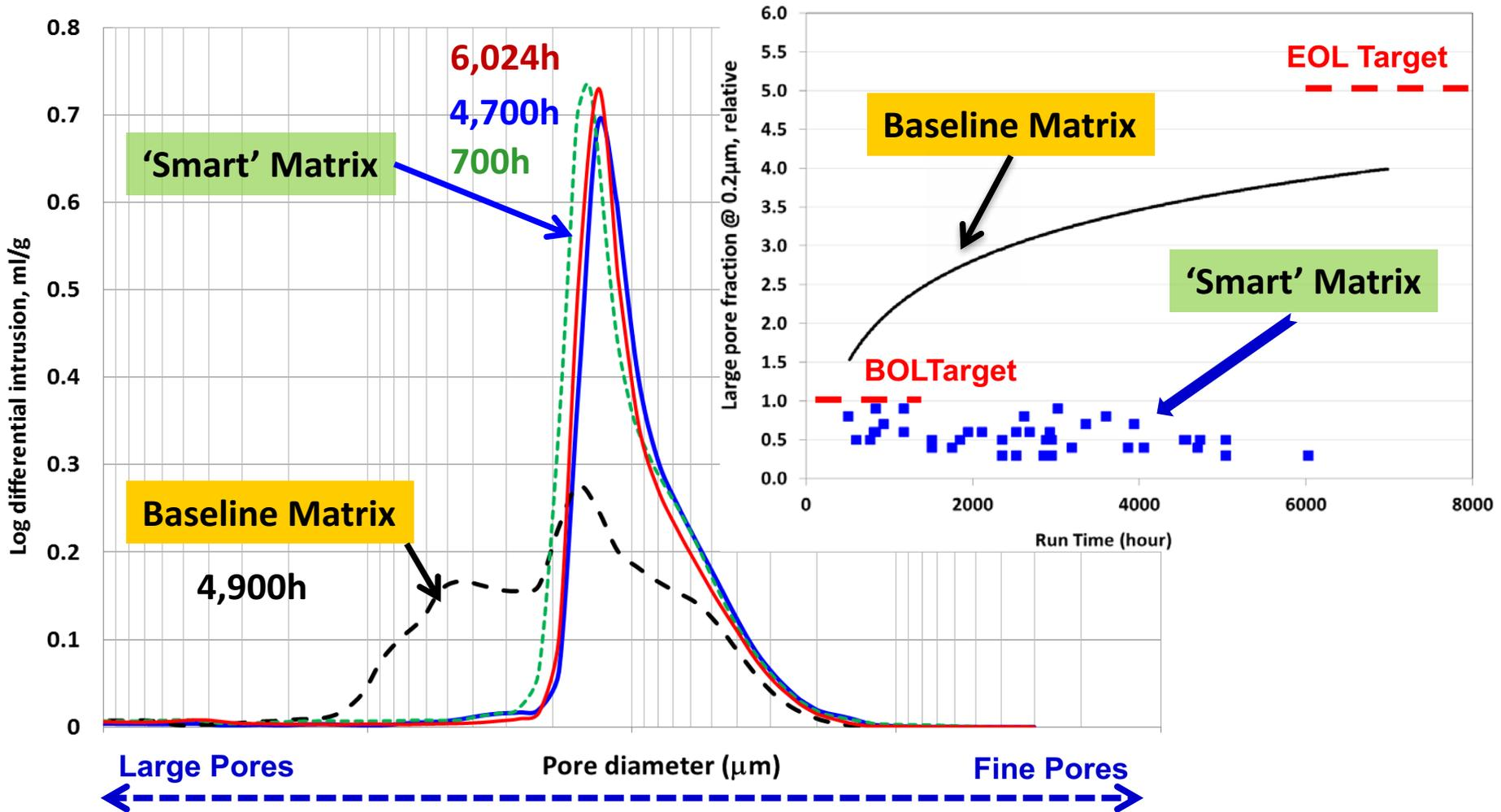
□ Projected meeting EOL\* pore-structure target (<50% of pores >0.2µm in 10 years) in accelerated cells
