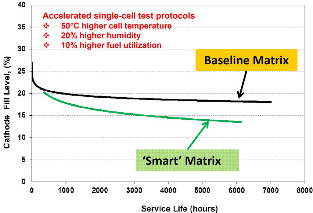
Reduced surface fine-oxide formation and ~40% reduction of Li consumption compared to baseline
