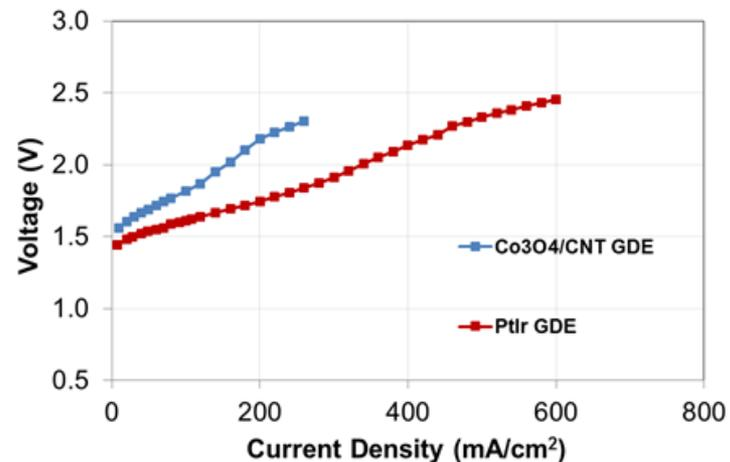
Anode are identical for all tests: PtRu/C (0.7 mg<sub>PtRu</sub>/cm<sup>2</sup>, I/C=0.8); Cathode: PtIr (0.75<sub>Pt</sub>+0.75<sub>Ir</sub> mg/cm<sup>2</sup>, Ionomer=20%); Co<sub>3</sub>O<sub>4</sub>/oCNT, 3 mg/cm<sup>2</sup>, 30% ionomer, Tokuyama A201 membrane, NREL Gen 2 ionomer, otherwise noted
