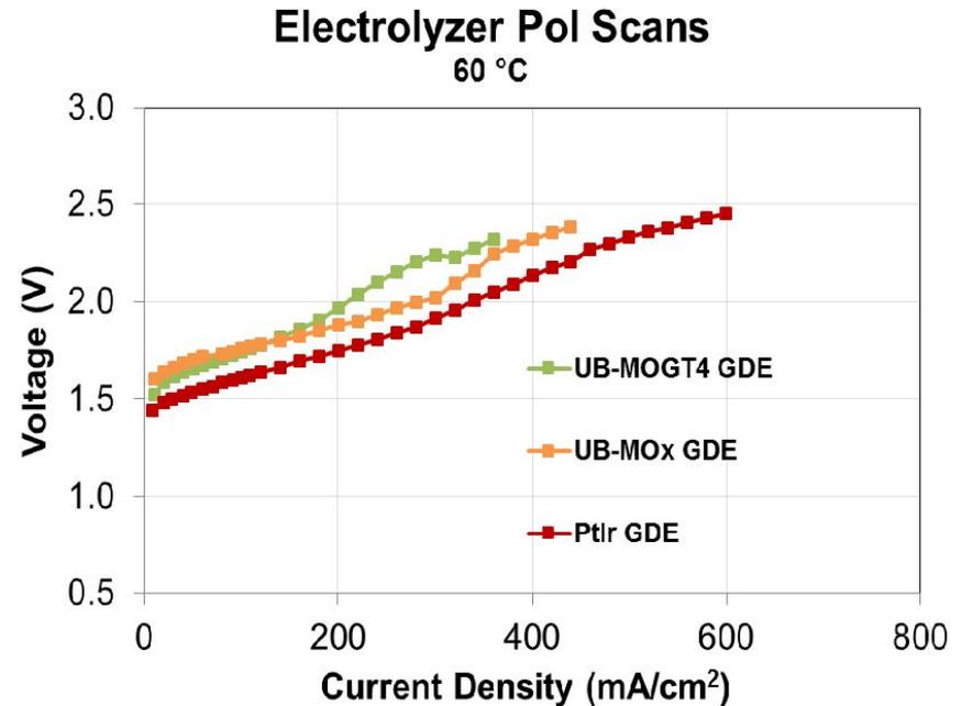
Fuel Cell test conditions: H<sub>2</sub>/O<sub>2</sub> flowing at 1000 ccm/min, at the temperature of 60 °C (relative humidity of 95%), and H<sub>2</sub>/O<sub>2</sub> backpressure of 30 psia
