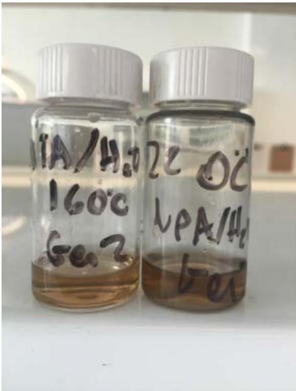
PFAEM Gen 2 polymer has been dispersed in n-propanol/water mixtures and successfully utilized as AMFC electrode binder
