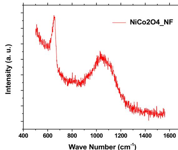
The XRD and Raman confirmed NiCo<sub>2</sub>O<sub>4</sub> phase and peaks for Nickel-Cobalt Oxide are well in agreement confirmation the formation of NiCo<sub>2</sub>O<sub>4</sub> phase.
