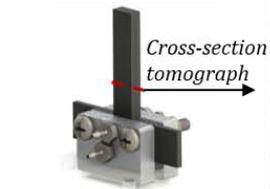
Assembled cell at the beamline stage
