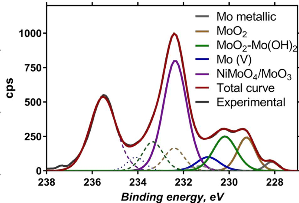
**Surface of catalyst is covered with Ni and NiMo oxides**
