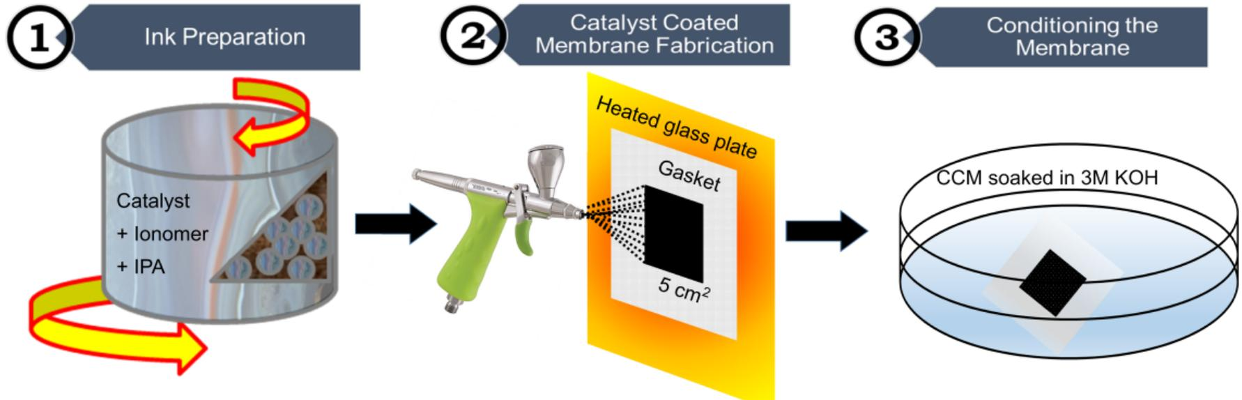
Mixture of catalysts, Tokuyama ionomer and alcohols were dispersed by ball-milling: 450RPM, t=20 min.
