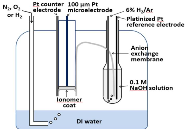
Microelectrode set-up for alkaline HOR study
