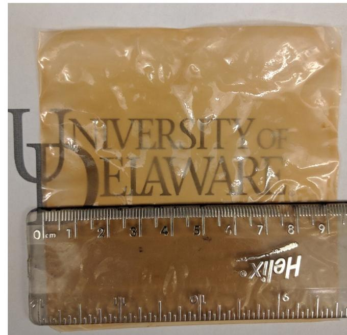
Picture of 9MeOTTP-PBI PTFE reinforced membrane
