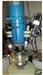
Hg/Hg<sub>2</sub>SO<sub>4</sub>, Salt Bridge
