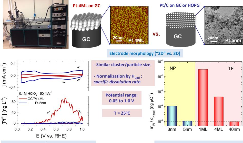
**3D** morphology of Pt/C layer over GC enables redeposition of Pt and attenuates dissolution
