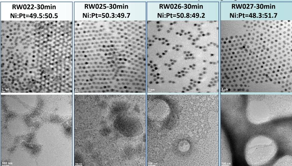
Desirable mono-dispersed 5 nm PtNi nanoparticles are obtained reproducibly
