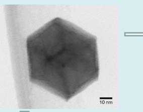
PtNi solid polyhedra are converted into hollow nanocages after evolution treatment
