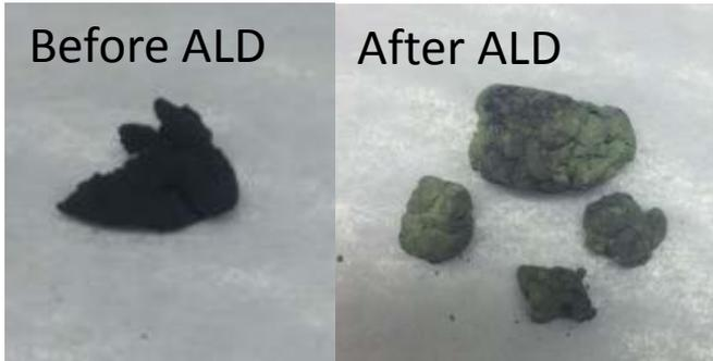
Dilute O<sub>2</sub> prevented excess oxidation, and resulted in improved properties/performance
