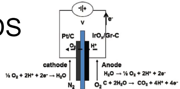
Figure 1. Schematic illustration of the experimental setup for the electrochemical measurement of the O<sub>2</sub> permeability through a polymer electrolyte membrane.
