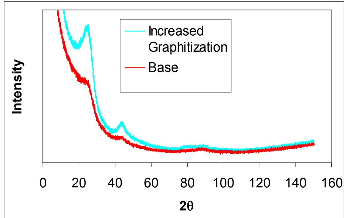
Higher graphitization leads to more corrosion resistance under Start-Stop AST protocol
