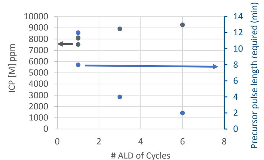
First ALD cycles fill micropores and deposit at higher growth rates. Subsequent cycles display consistent growth rates.
