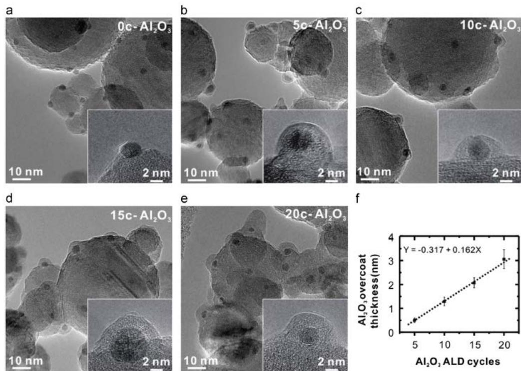
Pd:Al<sub>2</sub>O<sub>3</sub> catalysts with 0-20 Al<sub>2</sub>O<sub>3</sub> ALD overcoating cycles. [Lu et al., Surf Sci Reports 71 (2016) 410-472]
