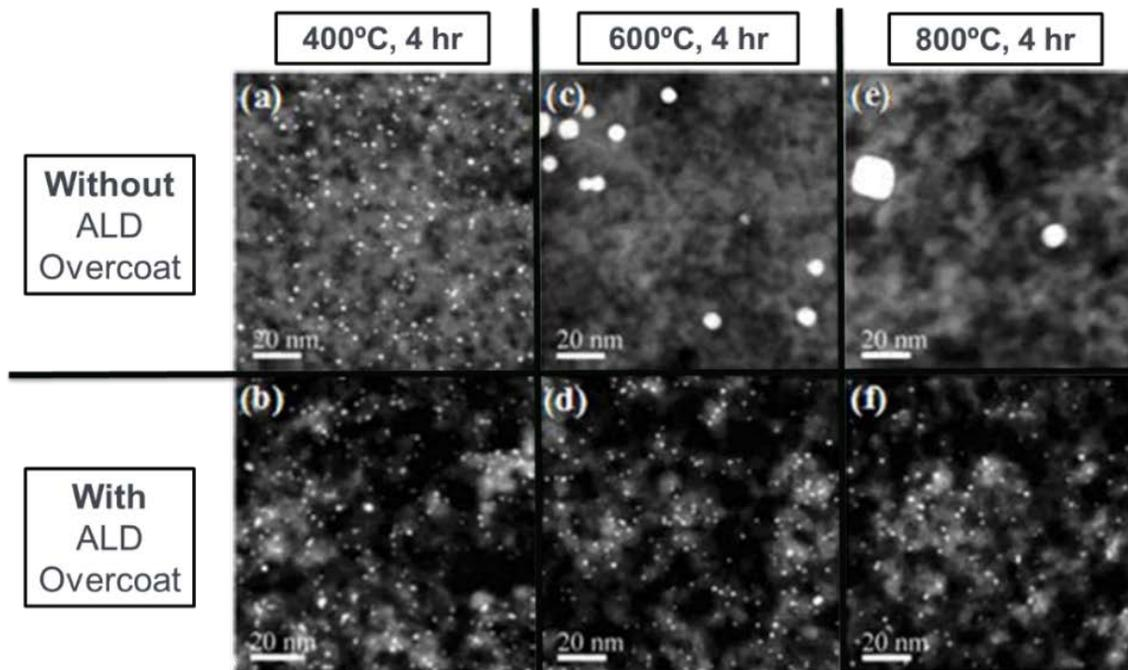
Al<sub>2</sub>O<sub>3</sub> ALD overcoating on ALD-derived Pt nanoparticles, showing effective elimination of sintering/ripening at high temperatures. [Liang et al. ACS Catalysis, 1, (2011) 1162-1165]
