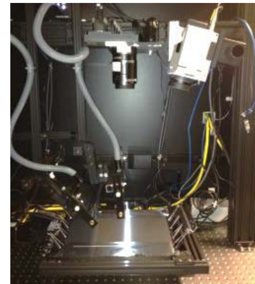
Thermal scanning configuration on optical testbed
