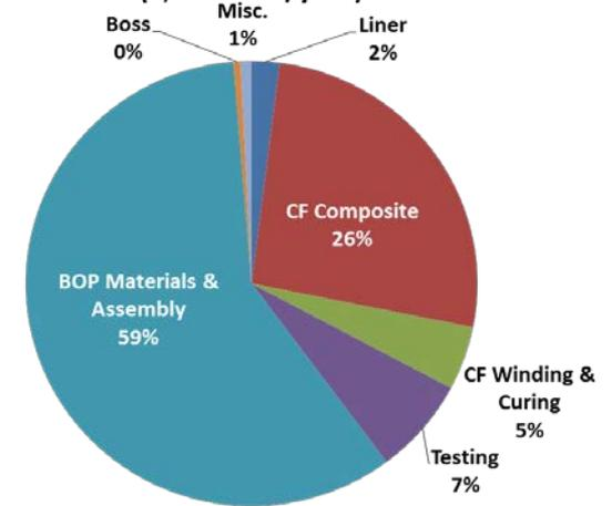
700 Bar Type IV Pressure Vessel Cost Breakdown (100,000 units/year)
