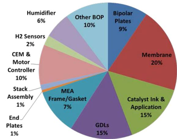
Fuel Cell Stack Cost Breakdown (100,000 units/year)
