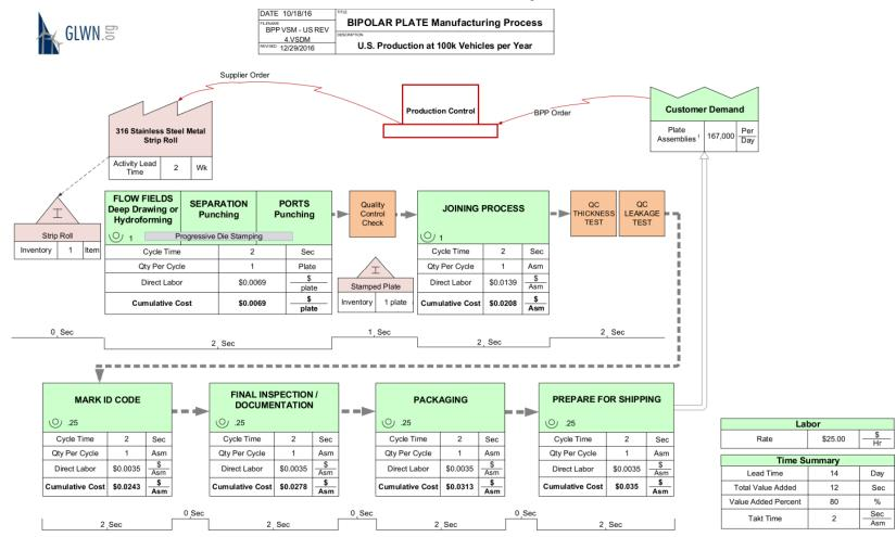
Value Stream Map is a hybrid of process flow used in DFMA and inputs from suppliers and OEMs VSM outputs are used for cost breakdown analysis and as a cost reduction tool
