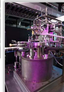
TAP reactor for extracting quantitative kinetic data
