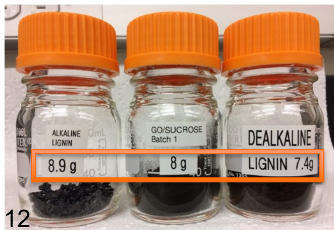
Figure 2. Left: Over 20 grams of graphene-based material was synthesized from reaction of graphene oxide with sucrose, alkaline lignin, and dealkaline lignin, the parameters for which are given in Table 1.
