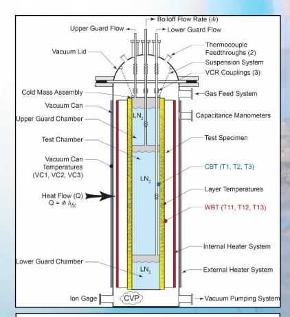
**Cryostat-100 Cylindrical Insulation Test Apparatus (Absolute)**
